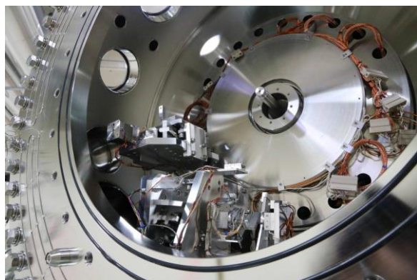
Figure 1: The TACoDE system with two principal rotation axes at the TPS.
