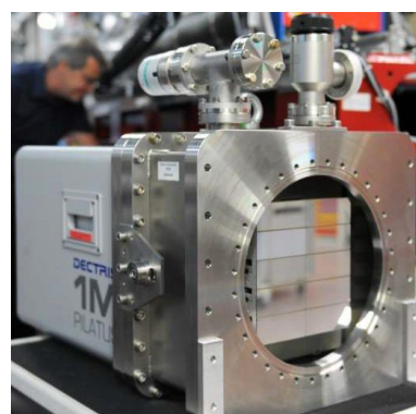
Figure 2: In-vacuum PILATUS 1M detector at the FCM beamline of PTB at BESSY II. Image courtesy of M. Krumrey (PTB).
