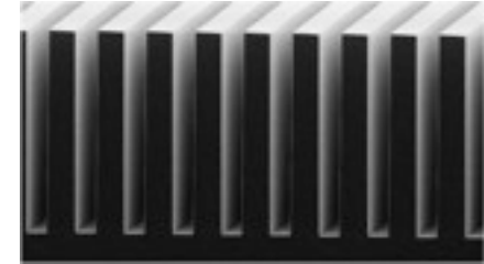
Si grating ( 4 \mu\text{m} pitch)
