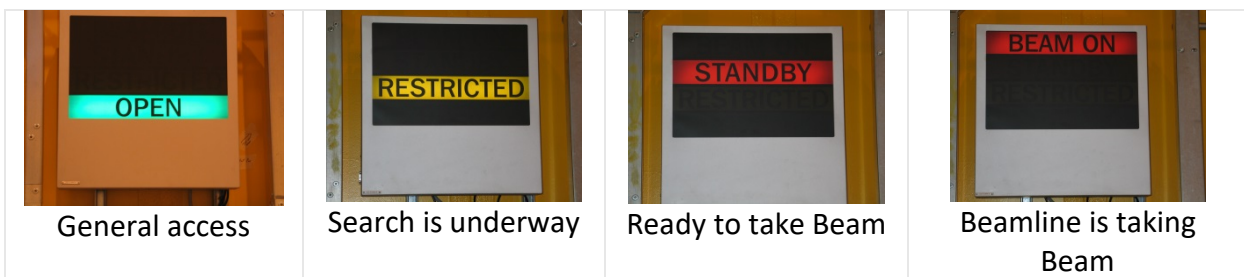
Fig 2 PSS annunciator displaying different stages in the beamline.
