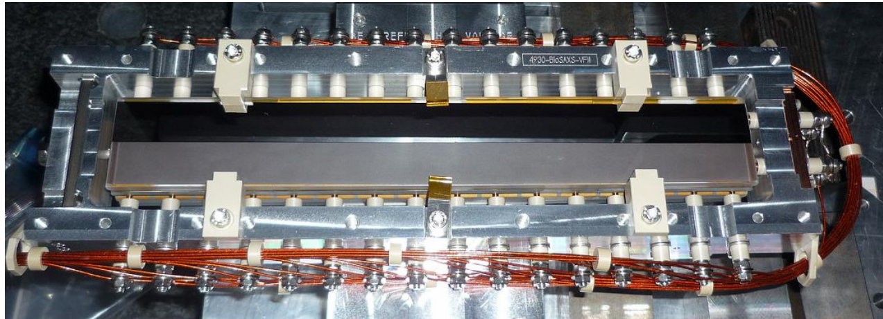
Bimorph-mirror with 16 electrodes BIOSAX-VFM for EMBL-Hamburg
