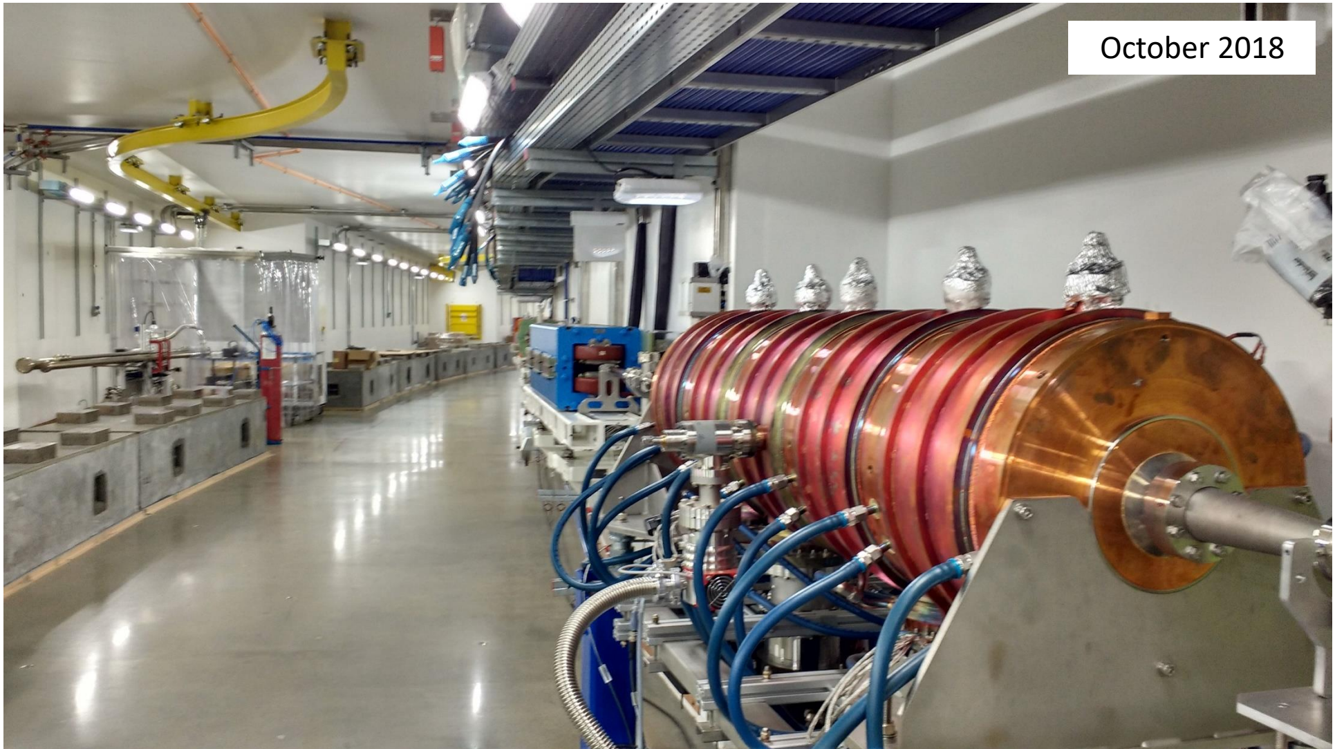
Booster cavity in place and e^- beam at 10^{-8} mbar
