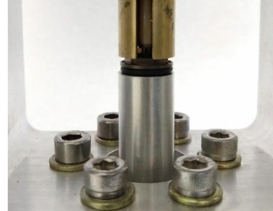
Force on separate feedthrough w/ leak detection
