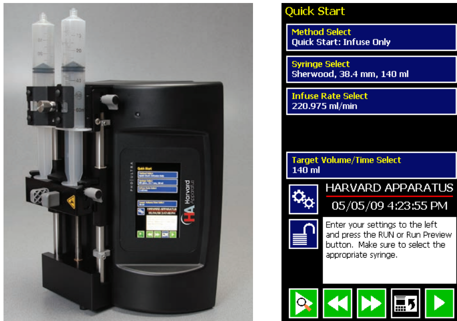
The PHD ULTRA™ pump shown in its vertical (upright) orientation and the associated Quick Start menu screen showing the application auto-rotated into portrait mode.
