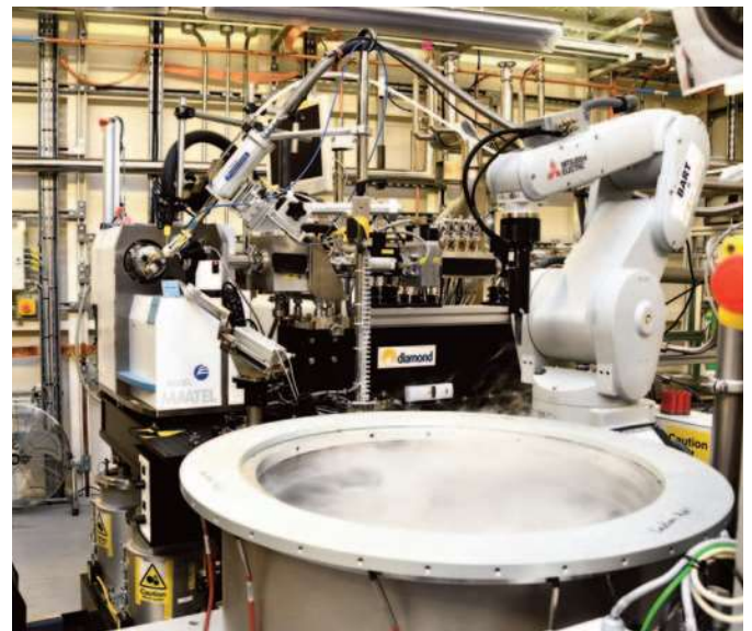
Beamline I04-1 Experimental Hutch - Sample changer and sample environment 2 – Copyright of Diamond Light Source Ltd.
