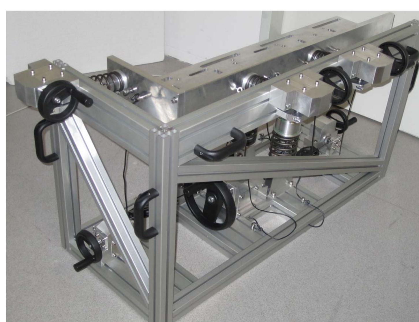
Figure 10: the alignment system (back view)
