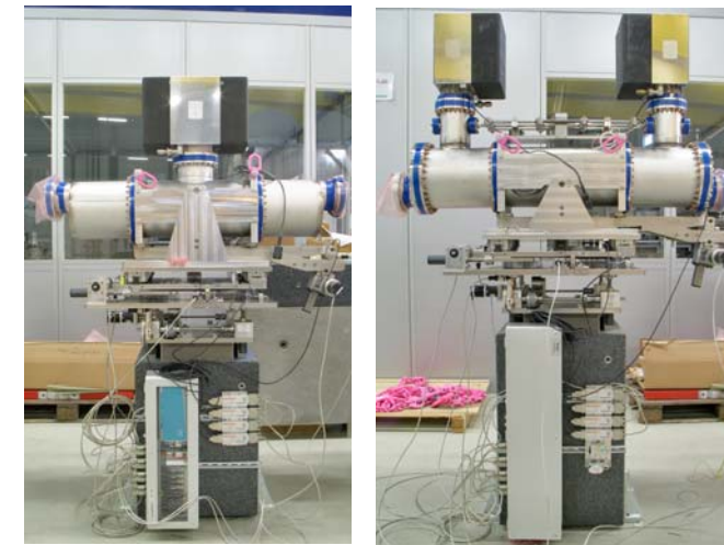
Plane mirror (left) and pneumatic bender mirror system (right) for PETRA III with external degrees of freedom for alignment and pneumatic bending. Inside the vacuum chambers 1m long partially coated fused silica mirrors with 3 optical surfaces each are mounted. These systems are installed and in operation at PETRA III beamline P09.
