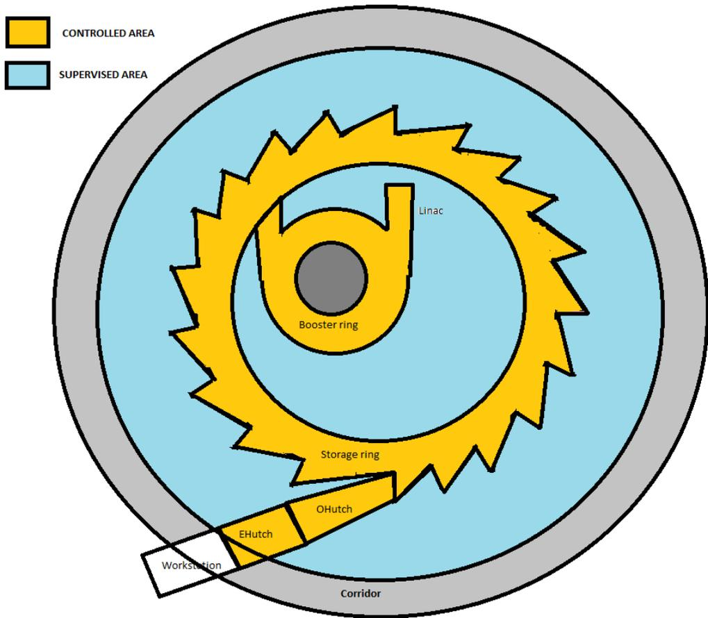
**Fig 3: Layout of controlled and supervised area in synchrotron ring.**
