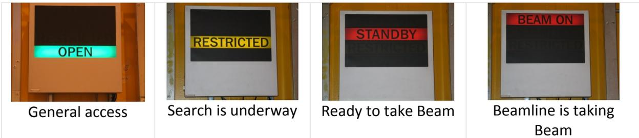
Fig 2 PSS annunciator displaying different stages in the beamline.
