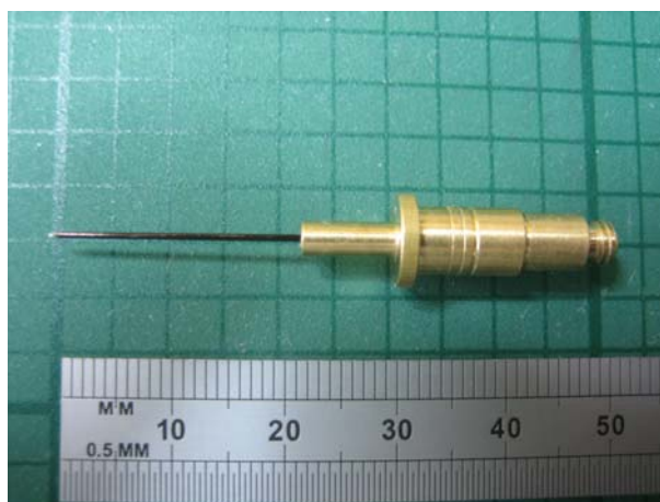
Figure 3. Loaded capillary attached to the brass tip ready for data collection
