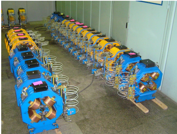
Quadrupoles and sextupoles for SR ALBA (250 pcs., France, 2008)
