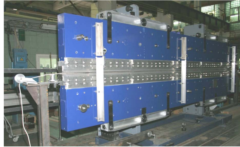
Undulator (prototype) for XFEL (Germany, 2014)
