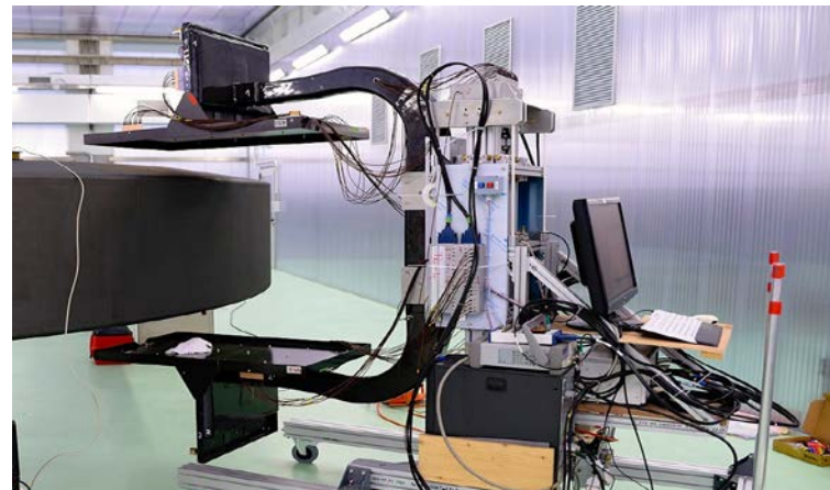
Field mapper to measure the first TF ITER coil
