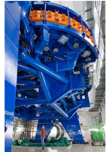
Heidelberg Ion Therapy, Carbon Ion Gantry 22m x 13 m , 600 tons (1/10 of the Eiffel Tower)
