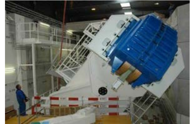
Proton therapy Gantry 2 (PSI) 8m x12m , 200 tons
