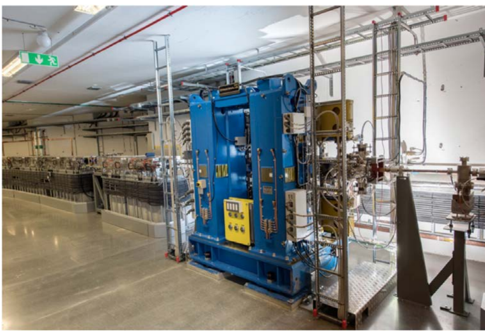
BioMAX in-vacuum undulator in ring tunnel
