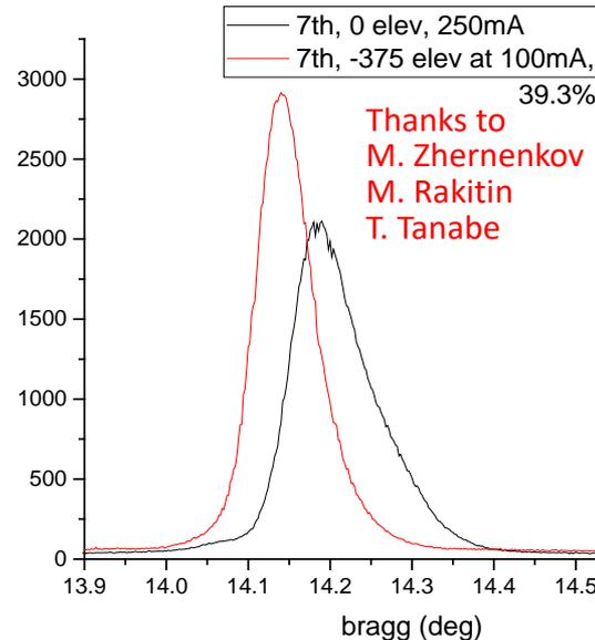
Spectral performance was ~fully restored by introducing -400  $\mu\text{m}$  change in elevation (the IVU was re-aligned mechanically then).
