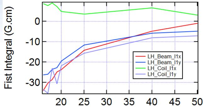
Integrated Field Integral variations with beam are larger than those by magnetic field measurement
