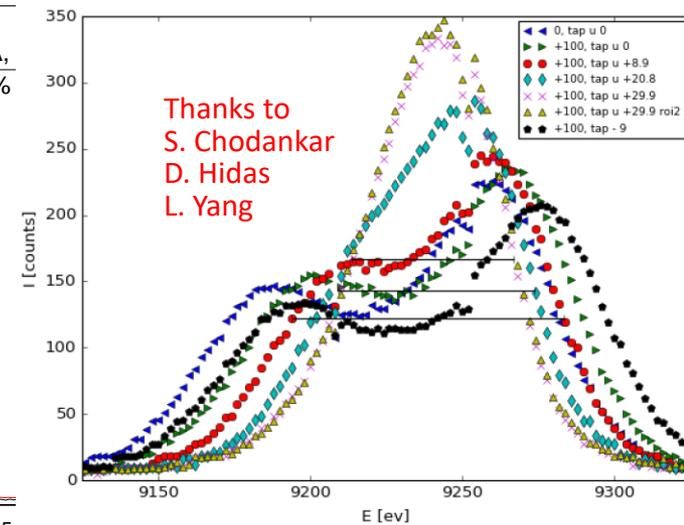
Spectral performance was significantly restored by introducing 30  $\mu\text{m}$  change in taper (work is still in progress).
