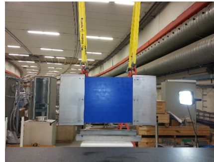
168 of those magnets assembled to a 2.6 t dipole for the n-ToF EAR2 experiment
