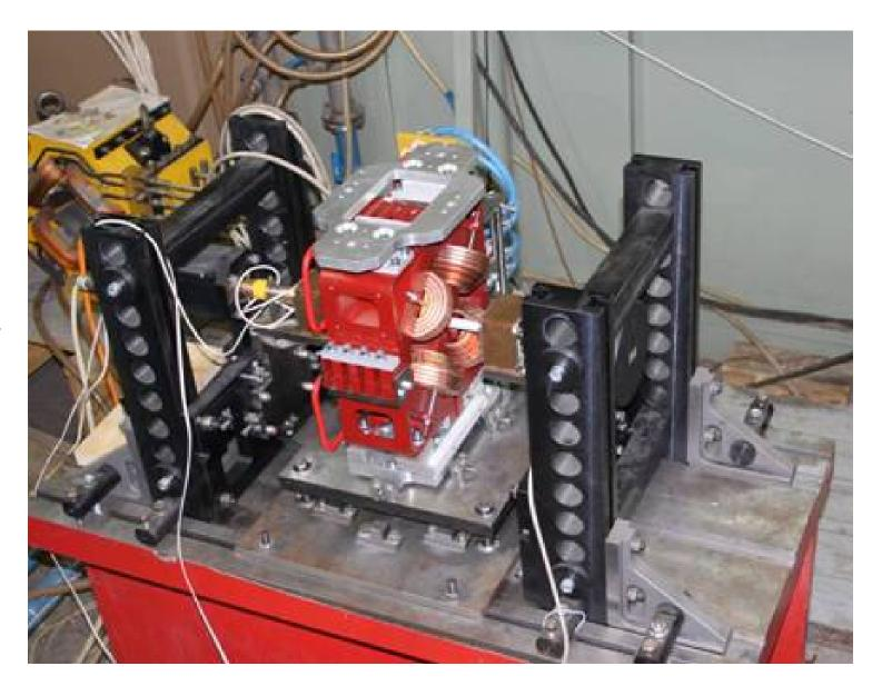
Rotating angle is done in fixed intervals. Measured by an angle encoder with an accuracy of  $2 \cdot 10^{-6}$ . For each rotation increment the voltage was measured. The dependence of the voltage signal from the rotating angle will be transformed in a Fourier series. Complete revolution -  $360^{0}$
