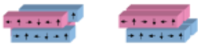
Figure 1. Shift modi of a fixed gap APPLE II: phase shift \phi with pairwise shifts of diagonal magnet arrays (left) and energy shift \rho with shift top versus bottom (right).
