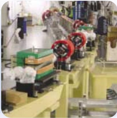
The electron beam is generated here in the linear accelerator
