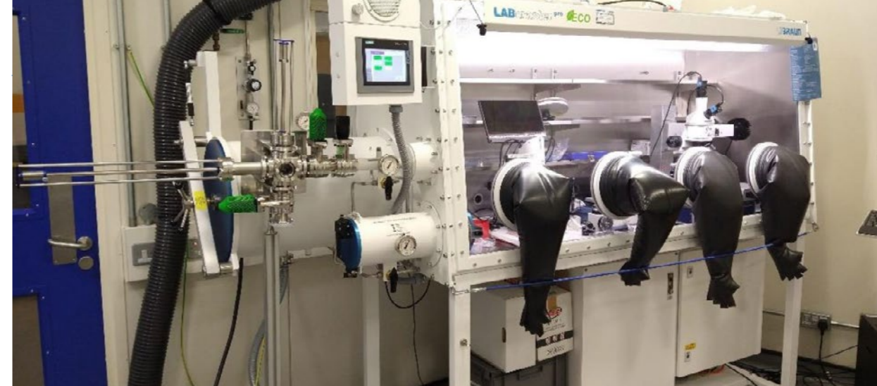
The recently installed glove box on beamline I05.
