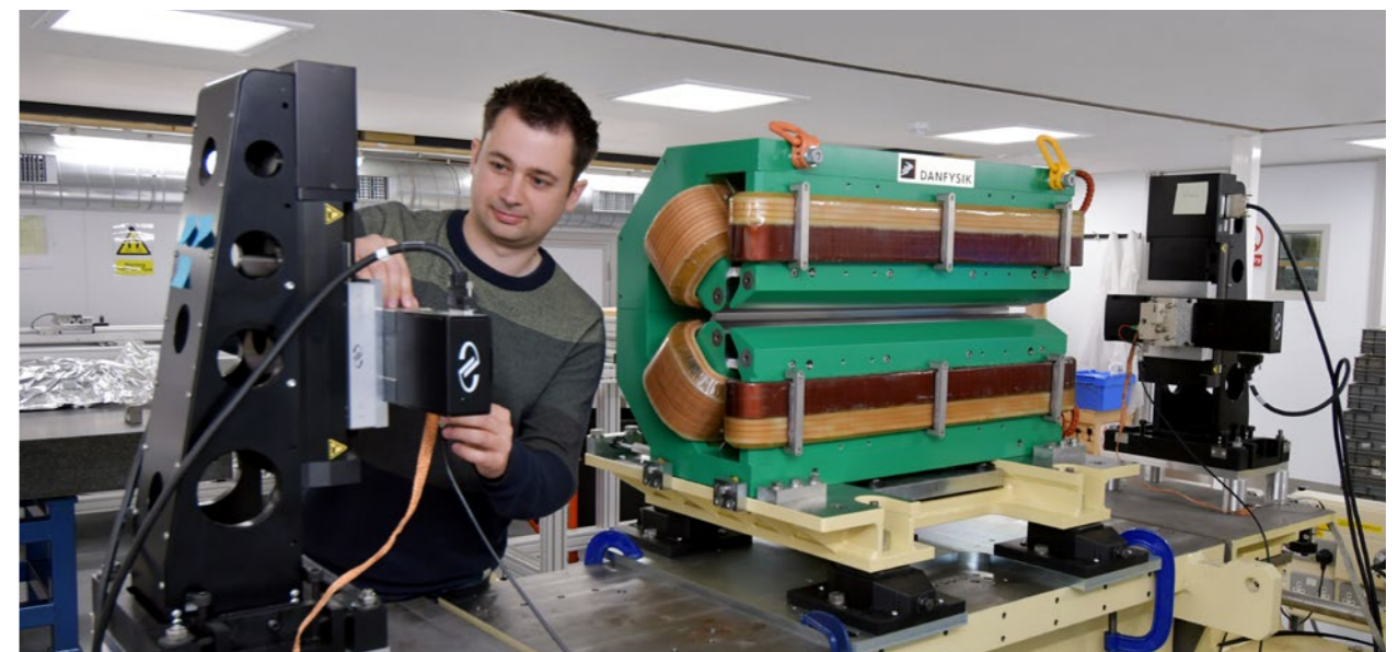
Figure 5. Prototype gradient bending magnet undergoing magnetic measurement using a stretched wire bench.
