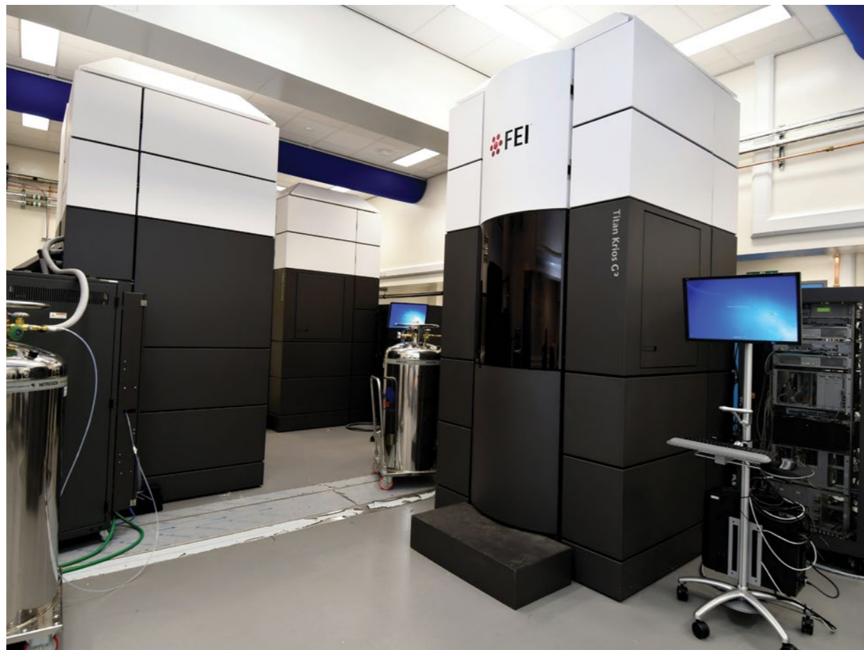
The Titan Krios is a state-of-the-art fully automated electron microscope designed for rapid, stable, high-resolution data collection on frozen-hydrated samples.
